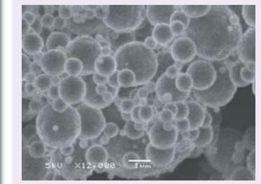
Scanning electron microscopy (SEM) image of particles of siRNA in a myo-inositol based formulation formed at 50 °C from a 10% aqueous solution (50 g/L siRNA, 50 g/L myo-inositol).
