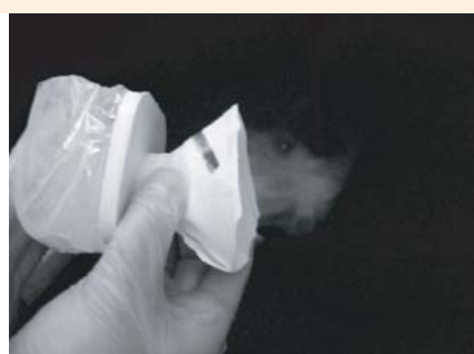
The PuffHaler active DPI, with valves and bottle aerosolizer (images at left), and detachable reservoir and mask with aerosolized dose being emitted (at right) upon gently squeezing the collapsible bag reservoir.
