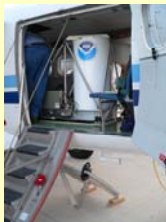
TOPAZ lidar mounted in NOAA Twin Otter
