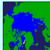
Figure 1. QuikScat egg field for 23 Jan 2000. In light blue are areas where ice occurred on all 5 days of the running mean (i.e., 21-25 Jan). White represents areas where ice was found on the surrounding four days, but not the 23rd. Red represents area where ice was found on the 23rd but not on any of the other four days. Note also the coverage extending only 60°N.
