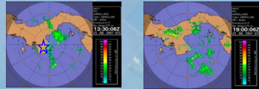
Figure 2. NASA NPOL radar scans at two time periods on July 21, 2007. The blue star identifies location of the DC-8 at 13:30 UT. Notice the difference between location of clouds between two periods of time. OMI overpass is at ~19:00 UT. The DC-8 location at 19:00 UT is outside of the lidar range.
