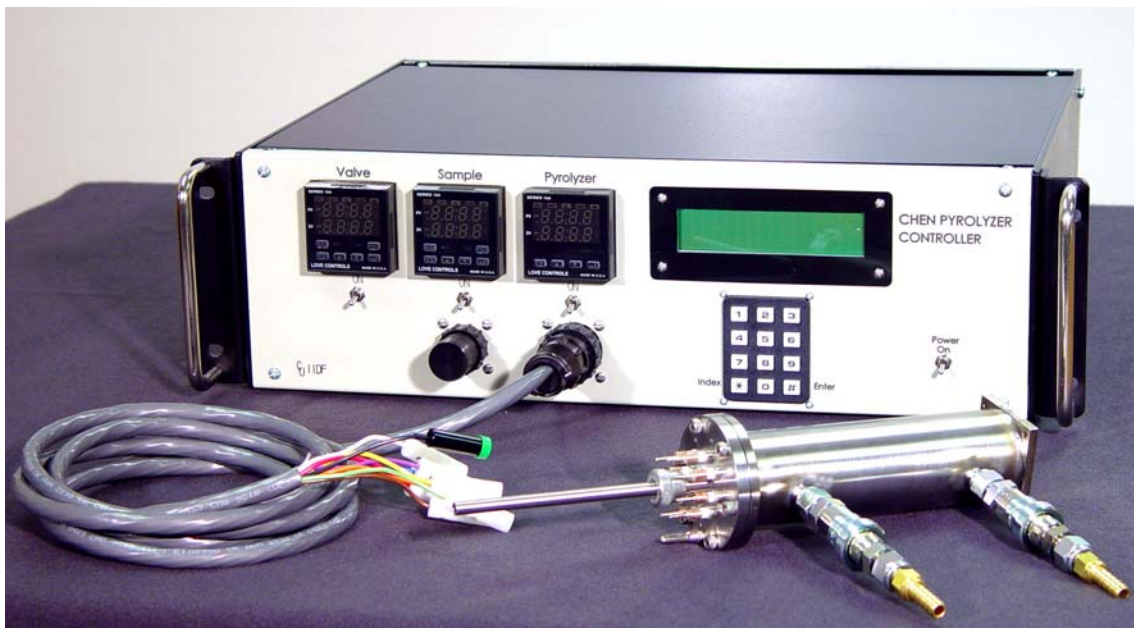
Figure 1 CU IIDF Pyrolyzer System
