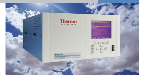
The Thermo Scientific Model 42i-TL Trace Level Nitrogen Oxide ( $NO_\chi$ ) Analyzer utilizes chemiluminescence technology to measure the amount of nitrogen oxides in the air from sub-ppb levels up to 1000 ppb.
