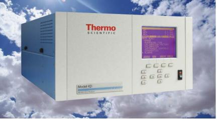
The Thermo Scientific Model 42i-Y NO<sub>Y</sub> Analyzer utilizes chemiluminescence technology to measure the amount of nitrogen oxides in the air from sub-ppb levels up to 1000 ppb.
