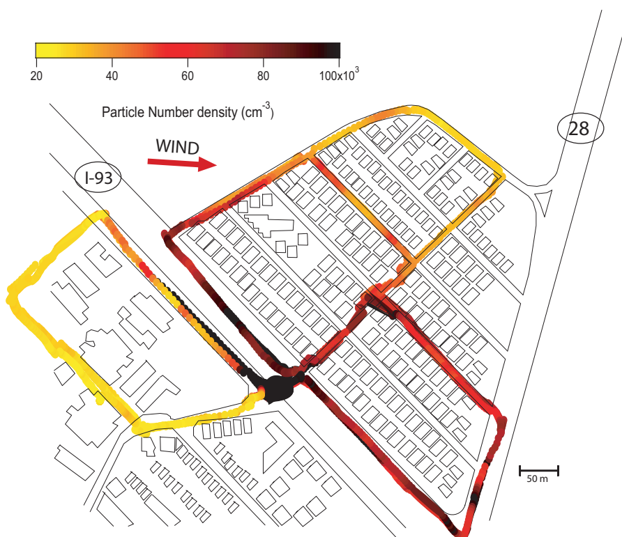
Figure 3. Particle number concentrations measured with a CPC downwind of major roadways and highways in Somerville, MA. These measurements were obtained with the Aerodyne mobile laboratory.
