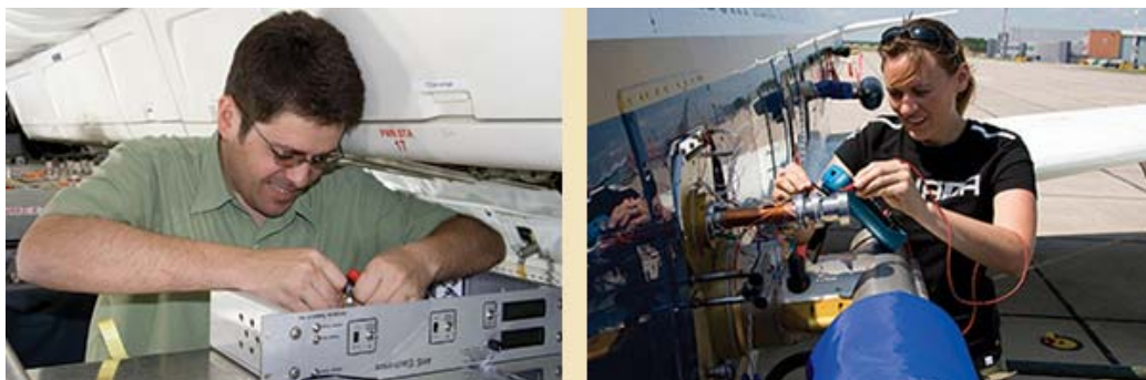
The aerosol mass spectrometer brought to ARCTAS by Jose-Luis Jimenez, left, (University of Colorado in Boulder) measured a record number of particulates. NCAR's Rebecca Anderson, right, carries out adjustments on an instrument from the DC-8 that measured hydrogen oxides. (Photos by Bob Henson.)
