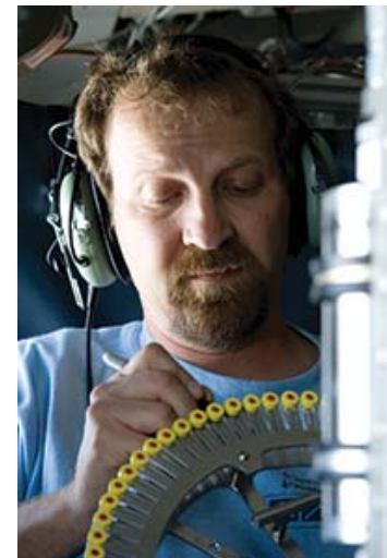
Rodney Weber (Georgia Institute of Technology) readies a set of sample vials that stored fine water-soluble particulates. These were collected during DC-8 flights for later analysis of a variety of aerosol properties. (Photo by Bob Henson.)
