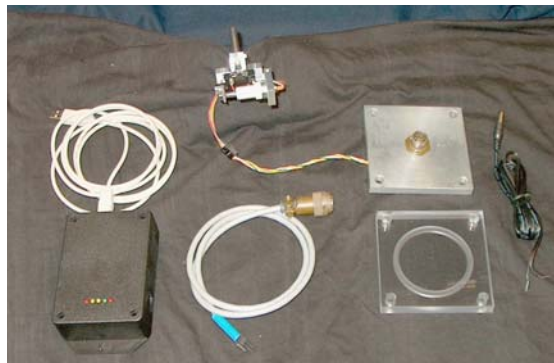
Figure 2. Beam Width Probe components.
