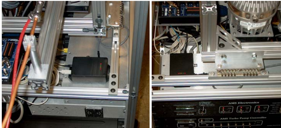
Figure 5. Suggested mounting location for the BWP control electronics.
