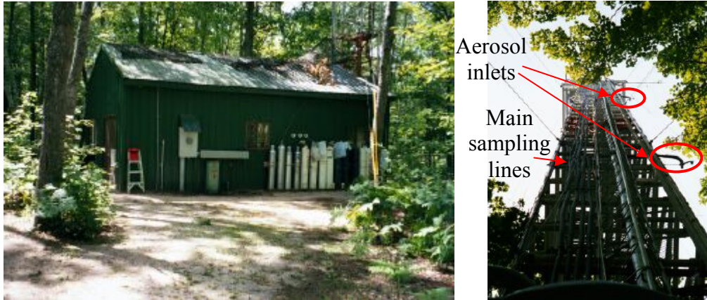
Figure 4.1: Picture of the PROPHEX laboratory building (left) with the base of the tower visible on the right side of the building and the tower (right) with the two lowest aerosol sampling inlets visible protruding from the right side of the tower.
