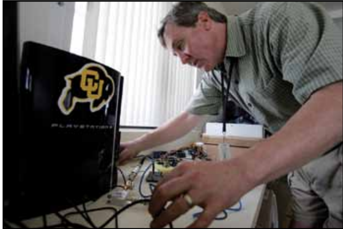
CIRES' Christopher Williams works on the prototype of his inexpensive vertical-profiling radar. The system uses a Sony PlayStation to process information captured by a set of three, $200 radar dishes.
