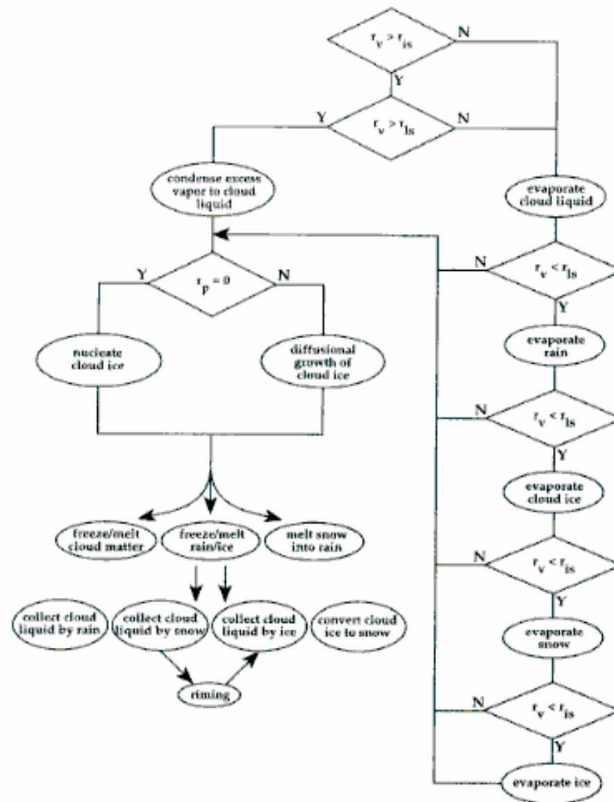
FIG. 1. Flow diagram for the NWP explicit microphysics algorithm; r is mixing ratio. The subscripts are v , vapor; p , cloud ice; ls , liquid saturation; is , ice saturation.
