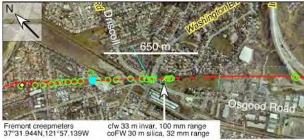
Fig. 14 Map and section for the Fremont Creep meters. Note there are two separate creep meters with different mounts and length standards (invar and silica). The measurements have detected the motion of a surface wedge in the uppermost 22 m of the fault zone. We are unable to make inclinometer measurements to detect tilt of the 30 m deep boreholes because of our request to purchase an inclinometer was declined by the USGS. A new road system is being constructed near the site and the transmissions have been twice vandalized possibly as a result of increased exposure.
