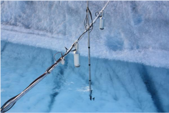
Figure 4. Gauging station set-up.
