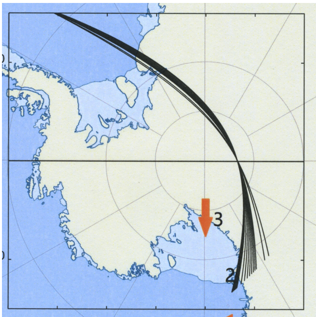
Figure 11: Projection of the ray paths from figure 10 on the ground. The wave-normal direction of the wave that was transmitted at an elevation angle of -89.288^\circ is 11.3^\circ clockwise from north as it passes above McMurdo Station. This is reasonable agreement with the azimuth angle of 11^\circ clockwise of north given by Chen et al. (2013). The ray paths are superimposed on a map of Antarctica.
