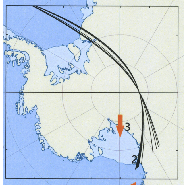
Figure 9: Projection of the ray paths from figure 8 on the ground. The wave-normal direction of the wave that was transmitted at an elevation angle of -89.416^\circ is 11.4^\circ clockwise from north as it passes above McMurdo Station. This is reasonable agreement with the azimuth angle of 11^\circ clockwise of north given by Chen et al. (2013). The ray paths are superimposed on a map of Antarctica.
