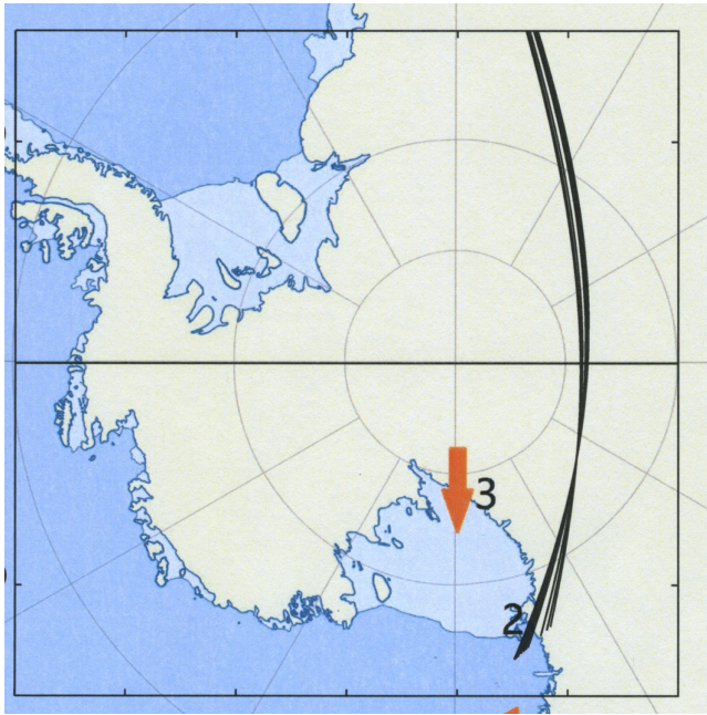
Figure 5: Projection of the ray paths from figure 4 on the ground. The wave-normal direction of the wave that was transmitted at an elevation angle of -89.349^\circ is 24.939^\circ clockwise from north as it passes above McMurdo Station. Moving the source location farther west would give agreement with the azimuth angle of 11^\circ clockwise of north given by Chen et al. (2013). The ray paths are superimposed on a map of Antarctica.
