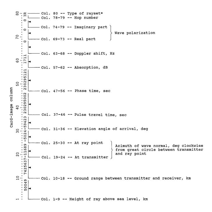
Figure 2.25. Definitions and format for a receiver rayset. \* type of rayset:  $G = bottom \ reflection$ ;  $M = closest \ approach \ to \ receiver \ height; <math>R = at$  receiver height;  $S = maximum \ number \ of \ steps$ ; E = extinction; F = exceeded maximum range;  $U = exceeded \ maximum \ height$ ;  $D = went \ below \ minimum \ height$ ;  $A = ocean-surface \ reflection$ ;  $X = bottom \ absorption$ ;  $A = implied \ decimal \ point$ .
