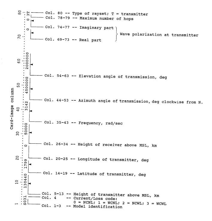
Figure 2.24. Definitions and format of a transmitter rayset.
