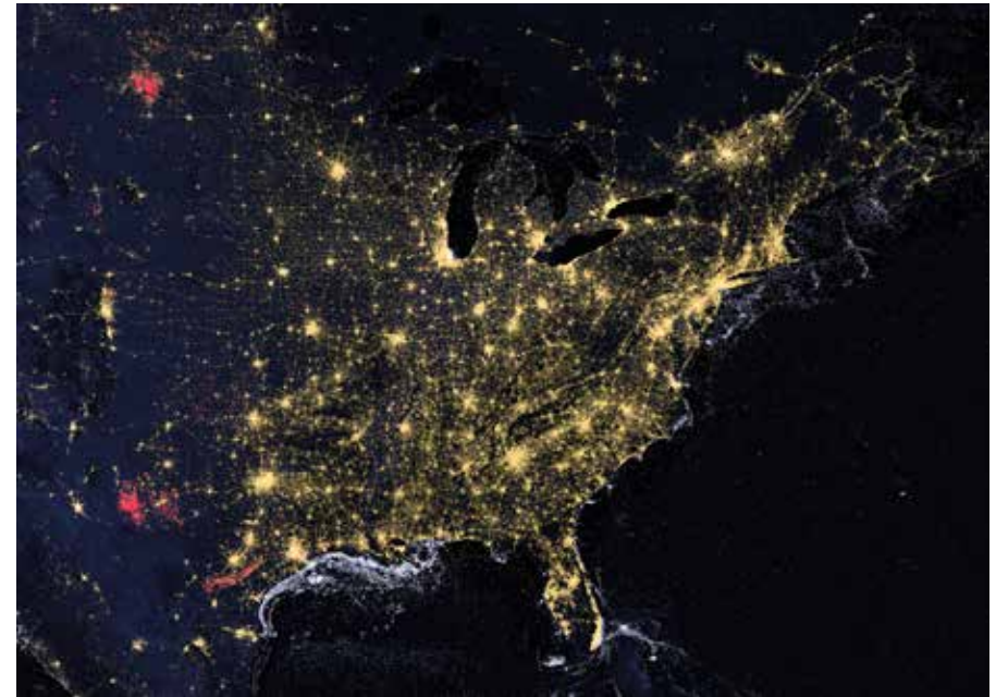
NCEI-07: Nighttime VIIRS product annual composite of the eastern United States. Stable lights are shown in yellow, gas flares as red, and boat detections in light blue, visually depicting the three VIIRS product lines, VIIRS Nighttime Lights, VIIRS NightFire, and VIIRS Boat Detection respectively. Image: CIRES/NOAA
