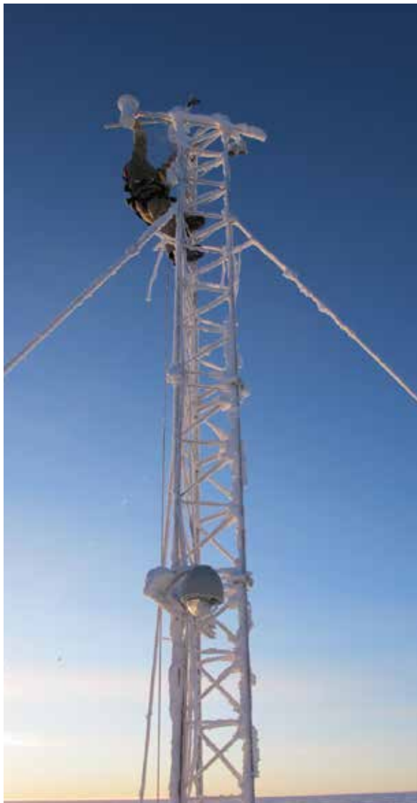
Cleaning frost from meteorological instruments on a 10-meter tower in Greenland. Photo: Sonja Wolter/CIRES
