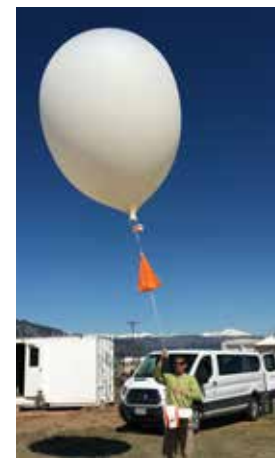
GMD-06: Emrys Hall (CIRES) prepares to launch a balloon-borne NOAA Frost Point Hygrometer, ozonesonde and radiosonde at the Marshall Field Site near Boulder, Colorado. Photo: Diane Perry/NOAA Corps
