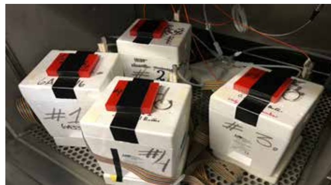
GMD-02, Fig. 2: Four ozonesondes installed in the environmental simulation chamber just prior to a simulation of an ozone sounding during a 2017 mission. Photo: Irina Petropavlovskikh/CIRES
