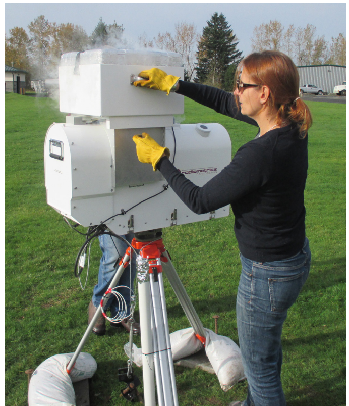
Liquid nitrogen calibration for the Radiometric Microwave Radiometer in Troutdale, Oregon. CIRES scientists in PSD developed a real-time, hourly-updated, online data product that helps forecasters at the Portland NWS Forecast Office monitor cool season easterly gap flow events to guide warnings to the public about potential weather-related hazards such as snow, freezing rain, and strong winds. Photo: Laura Bianco/CIRES
