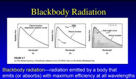
Greybody radiation —radiation emitted by a body that emits (or absorbs) with efficiency  $\epsilon$  (0 to 1.0) at all wavelengths  $\epsilon$  is called the EMISSIVITY
